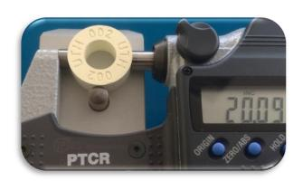
The temperature table provided for each UTH/UTL batch is a standard table and it is valid for 1 hour soaking time at peak temperature.
