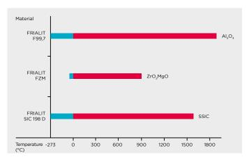
Operating temperature of FRIALIT-DEGUSSIT materials applied in oxidizing atmosphere
