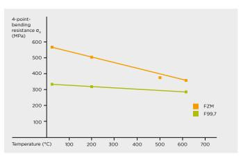
Bending resistance in relation to temperature
